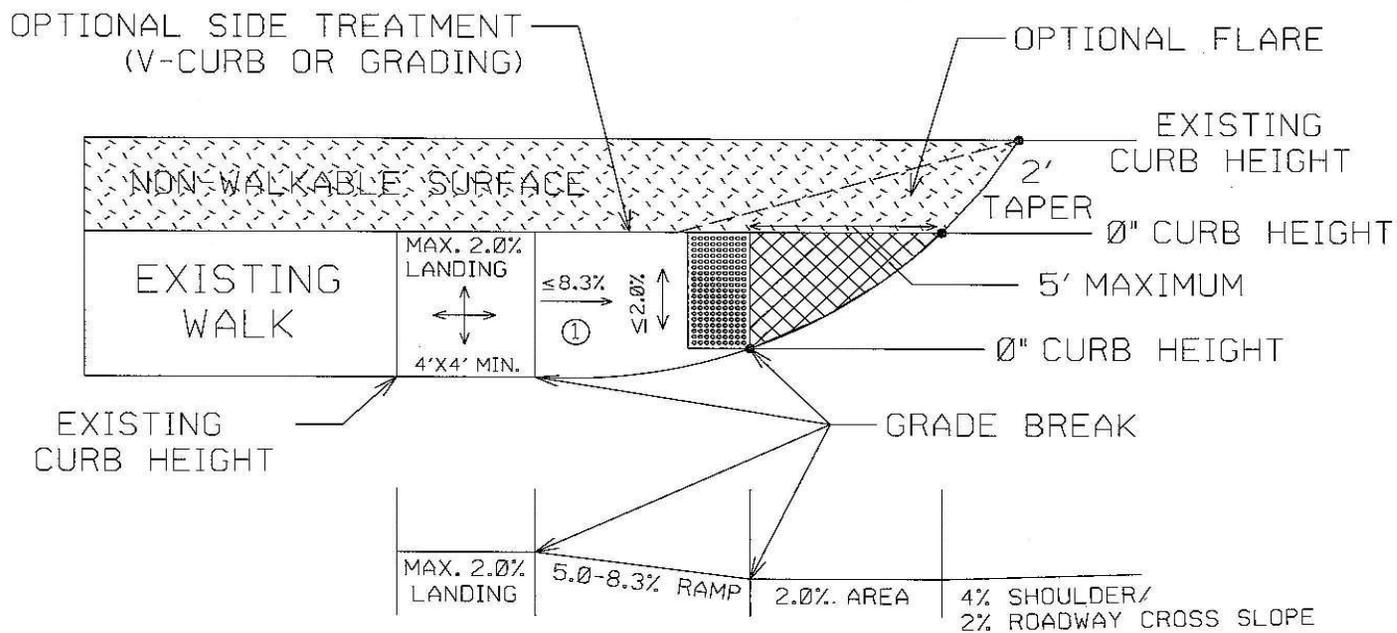
① IF RAMP SLOPE IS LESS THAN 5.0%, THEN NO LANDING IS REQUIRED.
