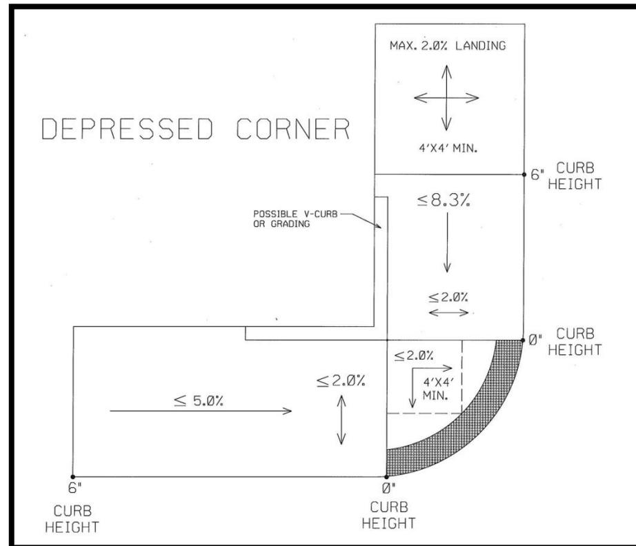
**Figure 8: Depressed Corner Detail**
