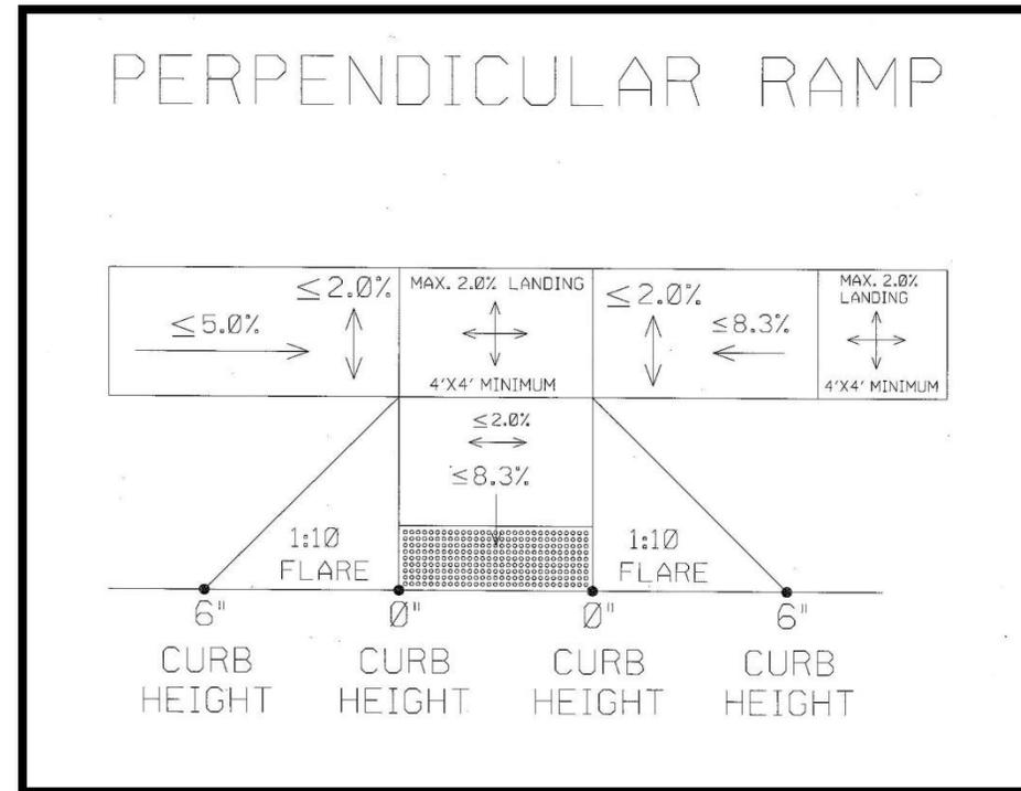
Figure 2: Perpendicular Ramp
