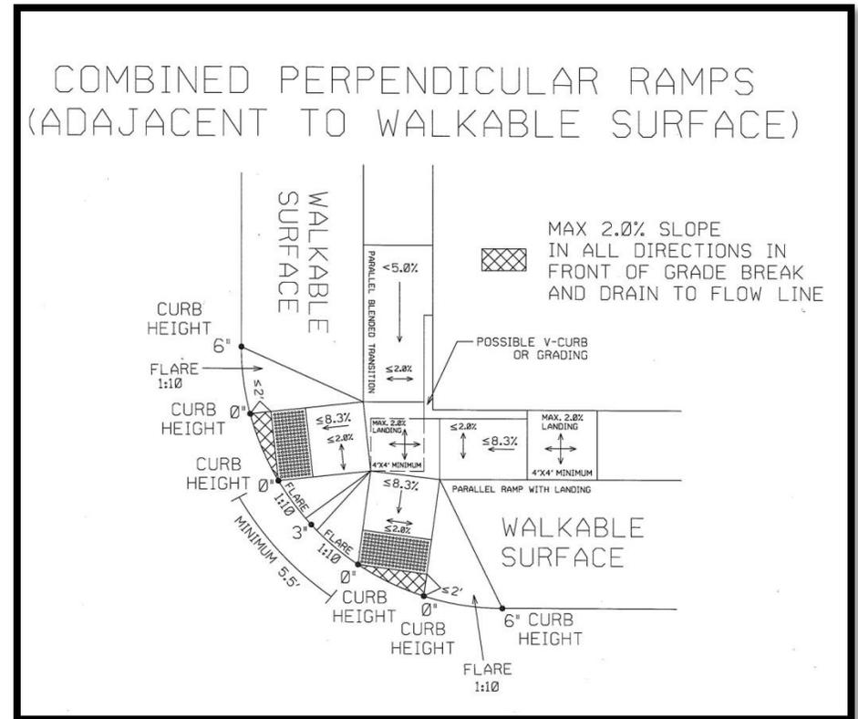
Figure 3: Combined Perpendicular Ramps Adjacent to Walkable Surface
