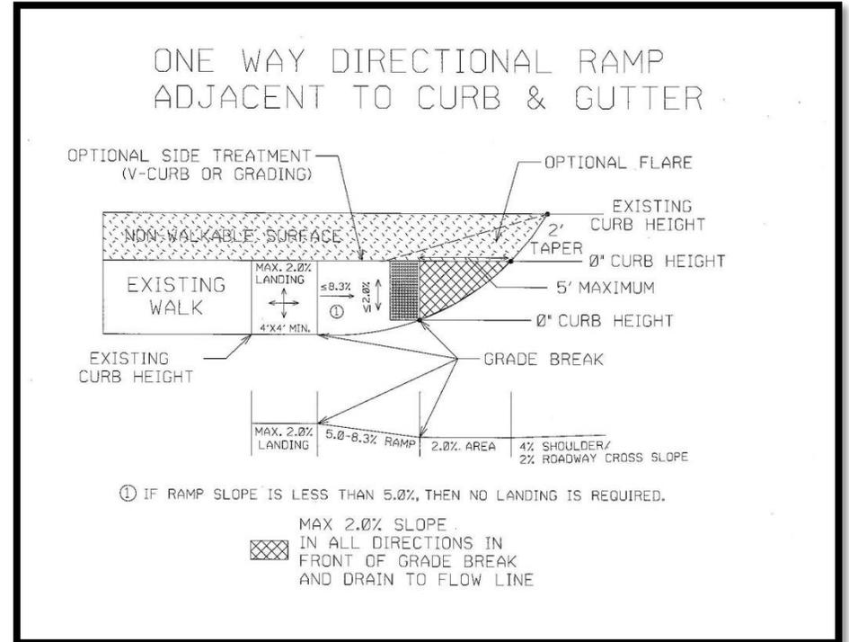
*Figure 5: One Way Directional Ramp Adjacent to Curb and Gutter*
