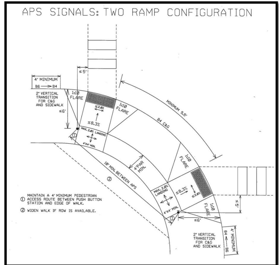
**Figure 14: Accessible Pedestrian Signal**
