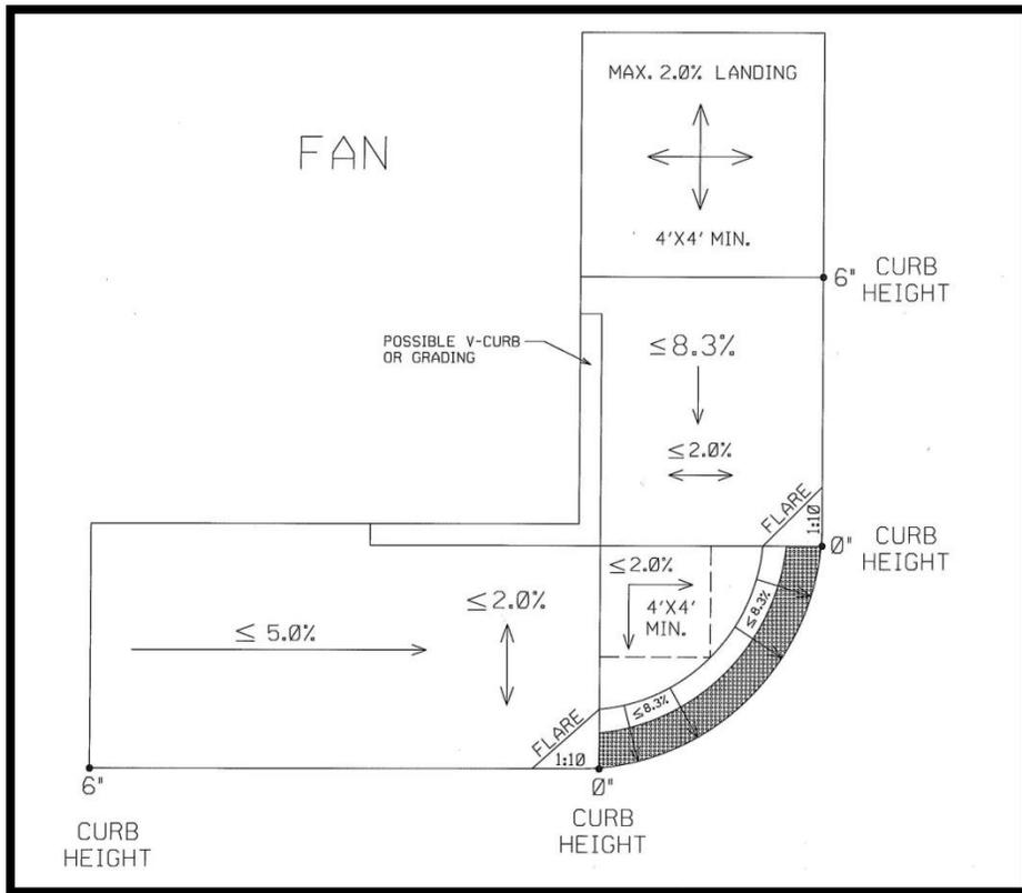
**Figure 9: Fan Detail**
