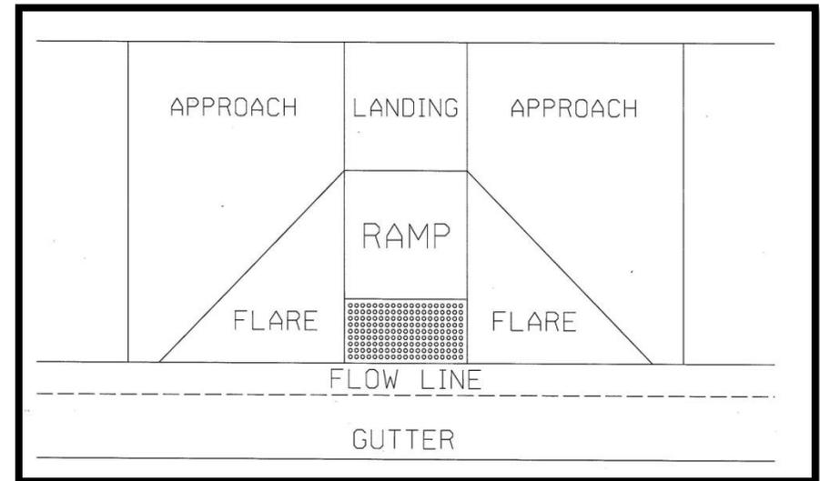
*Figure 1: Curb Ramp Components*
