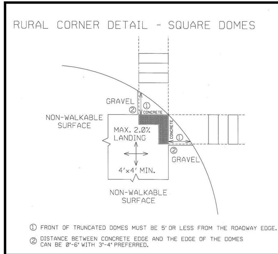
**Figure 15: Flat Landing with Directional Domes**
