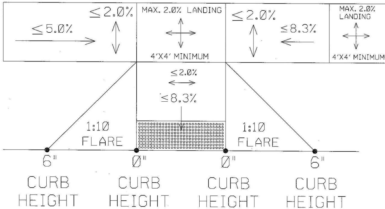
Figure 3: Combined Perpendicular Ramps Adjacent to Walkable Surface
