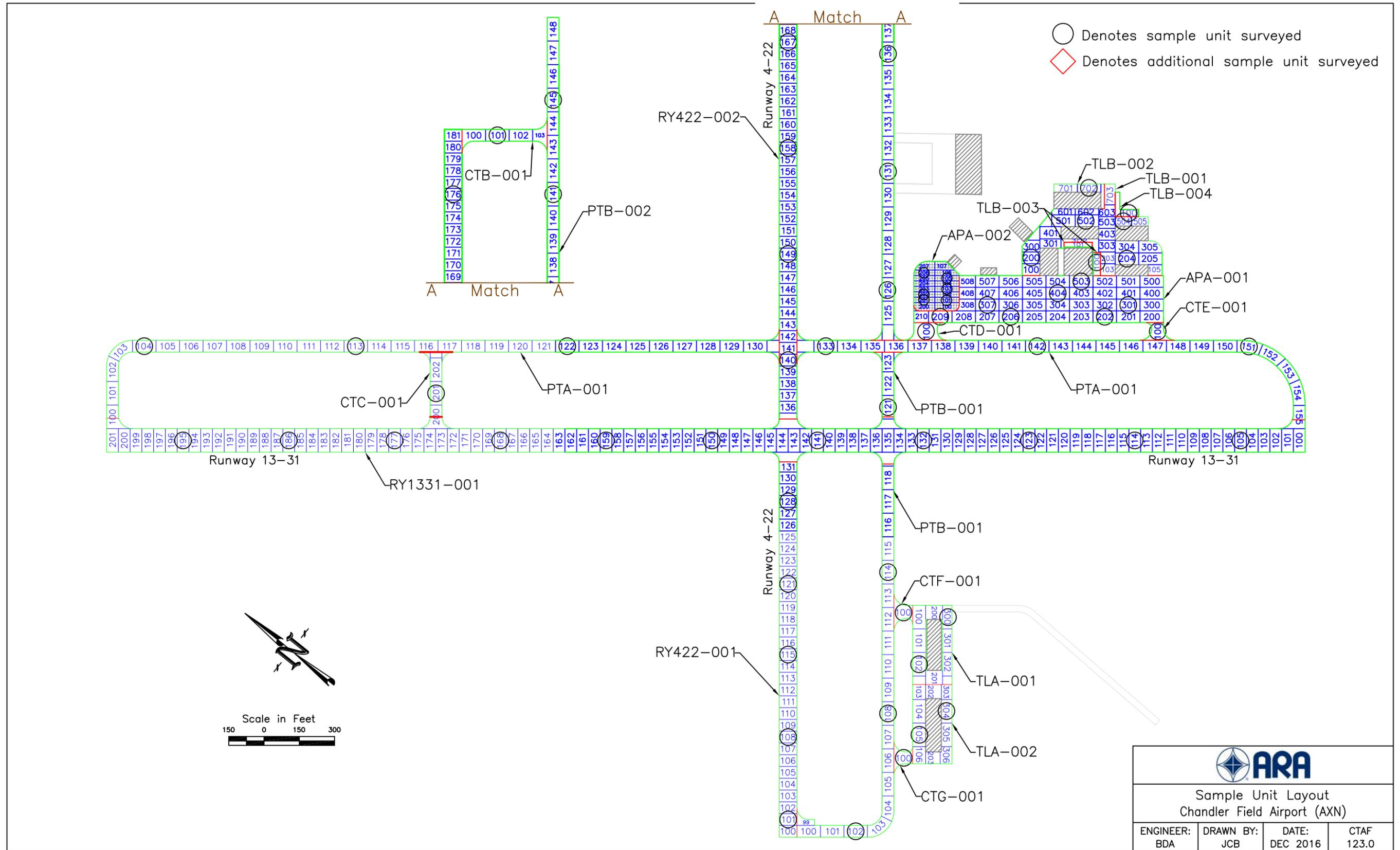
Figure A.1. Sample unit layout map at Chandler Field Airport (AXN).
