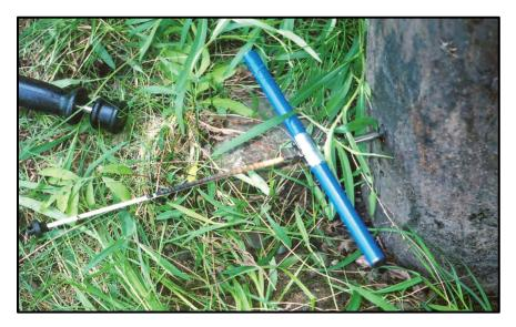
Figure 6.1. An increment core can be used to conduct inspections of timber bridge elements. This image shows an extracted core from an in-service timber pile ready for examination.
