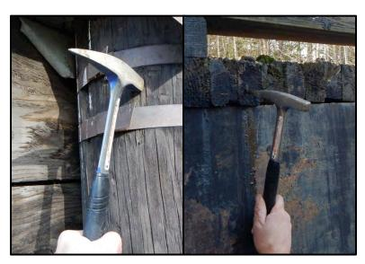
Figure 4.1. A hammer pick is an effective tool for initial assessments of timber bridge elements.
