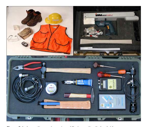
Figure 2.1. Inspection equipment used for inspecting timber bridges.
