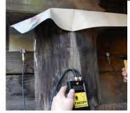
Typical areas of concern are below the cap, at water line and slightly below water line. Waterproof transducers are available.
