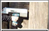
Resistance drilling can be used independently or to confirm stress wave testing results.
