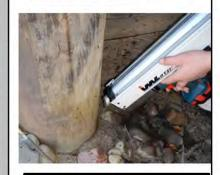
A 45° attachement allows for inspection below the water or ground line. Silicone should be used to fill the hole.
