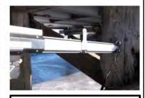
Press the drill firmly against the member, and press the start trigger, hold firmly until the drill reverses the bit out
