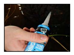
Figure 6.7. Silicone is used to fill the small drilling hole.
