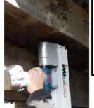
Vertical testing can be completed on timber caps or slab span members.
