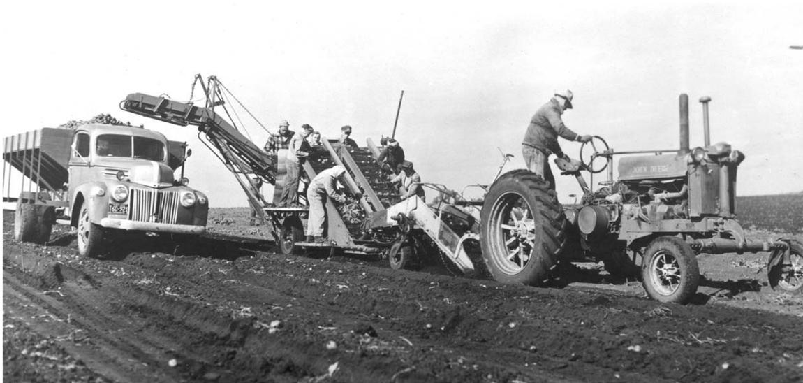
It was not until the 1940s that potato harvesting equipment became reliable. Before this time, most potatoes were brought to the surface with a potato plow. Machines like these led to the enlargement of fields and farms, and to the reduction of the state's farm labor force. Polk County, 1959. (MHS photo)
