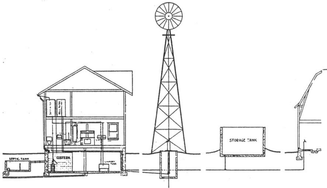
The position of the water storage tank within a typical farm water system, drawn by the University of Minnesota's Division of Agricultural Engineering. If the water tank was elevated, it could only be used for about seven months in Minnesota, but University staff pointed out that those seven months were busy on the farm and an elevated water tank might be well worth the investment. From Shepperd and Stewart's "Low Cost Water Systems for Farm Homes" (1922).
