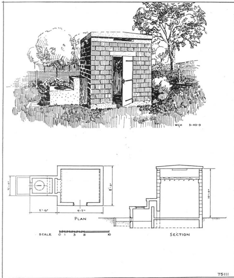
Designed by agricultural engineers for a plan catalog published in 1937, this smokehouse could be built of hollow tile or concrete block. Its floor, roof, and firebox were poured concrete. The 10'-tall smoke room measured about 8' x 9', while the firebox extension was about 4' x 5'6". From Midwest Farm Building Plan Service catalog of plans (1937).
