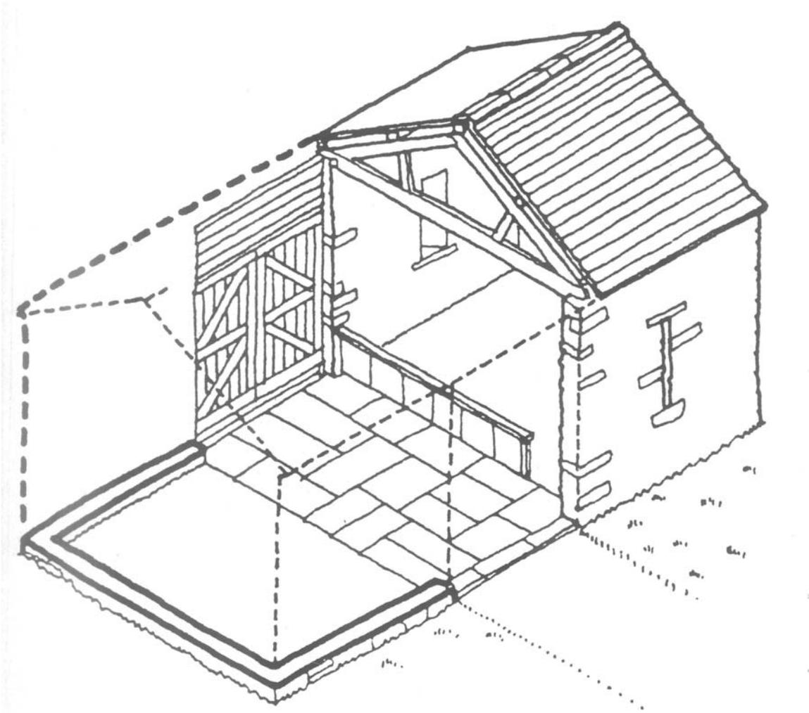
The anatomy of a three-bay threshing barn, which was usually supported by four bents. The central drive doubled as the threshing floor. Stored in one flanking bay were grain sheaves waiting to be threshed. Stored in the other bay were the products of threshing – the grain and the wheat straw. Animals were usually not housed in a threshing barn, and they did not have basements. From Calkins and Perkins, "The Three-Bay Threshing Barn" (1995).
