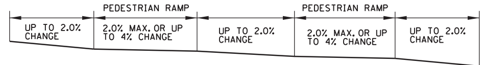
FLOW LINE PROFILE "TABLE" - TWIN PERPENDICULARS
