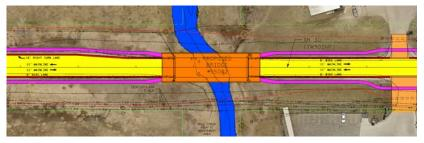
Bridge 9009 over the North Branch of the Root River will be replaced with a wider bridge to meet current design standards for shoulder width.
