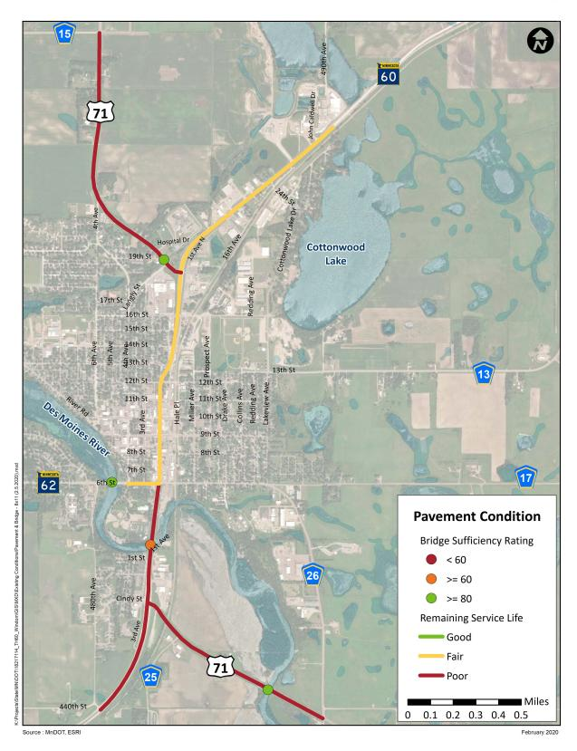
Figure 2: Pavement Condition and Bridge Sufficiency Rating
